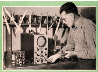
Here Arden is using a cathode-ray oscillagraph to measure the efficiency of one of his power plants. Such tests have shown that his latest product, which weighs only an eighth of an ounce, is more efficient, for each cubic inch of cylinder space, than the best modern two-cycle motor-boat engines!
